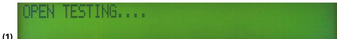
If it is having an OPEN circuit, find out which Address or Date is wrong according to the shown information.
