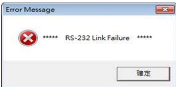
Please make sure the power of the Smart I/O is switched on before entering the system, if not, the image on the left will be shown:
